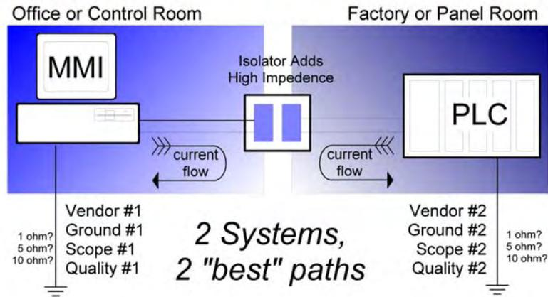
*Galvanic isolation breaks the ground path by using air-gaps, transformers, and/or optical devices. Galvanic isolation allows data to flow between systems, but not electrical current.* This protects your equipment, your warranty repair budget, and your reputation.
