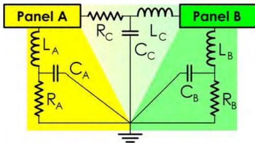
Another way to view the problem is shown at left. With 2 panels (whether 1 or 2 vendors) you have subtly different electrical characteristics on the ground/earth wire. Here we have inductance ( $L_A$ ), resistance ( $R_A$ ), and capacitance ( $C_A$ ) from panel A to site ground. We also have  $L_B/R_B/C_B$  for panel B and  $L_C/R_C/C_C$  on the data communication line between the 2 panels. So the question is - "during a surge or ground fault
