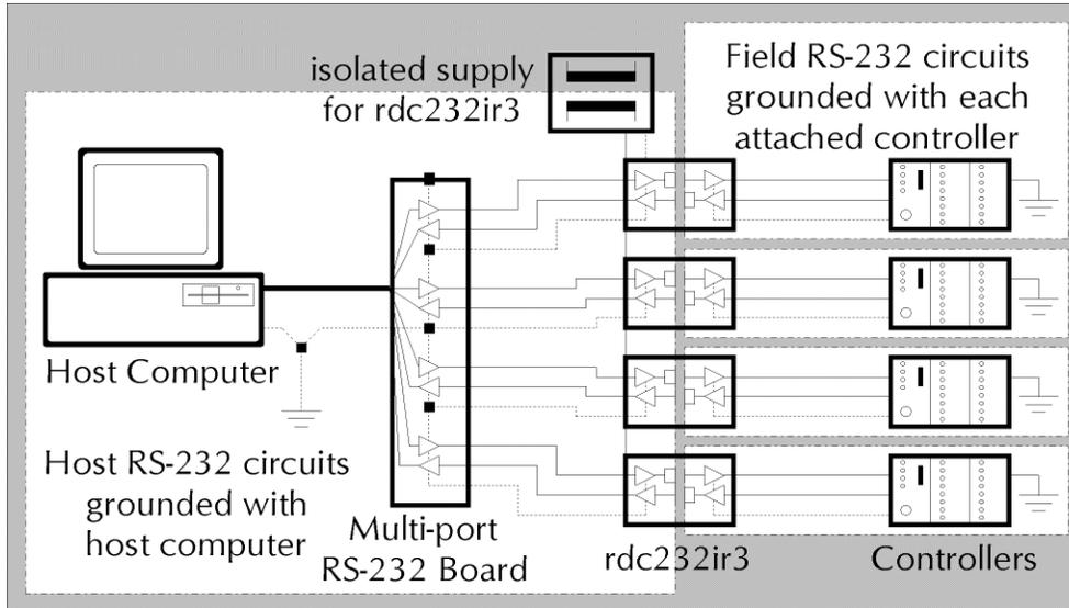
Here is a common installation of the rdc232ir3 with 2-port galvanic isolation. A small power supply with 1Kv isolation powers the four rdc232ir3 units. Since all four host RS-232 circuits share a common ground within the computer, any concern
