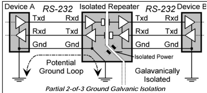
2-port isolation does present another problem; if the isolated repeater shares a DC power supply with other devices, then faults creating surges in the common power supply could effect device A through the isolated repeater.
