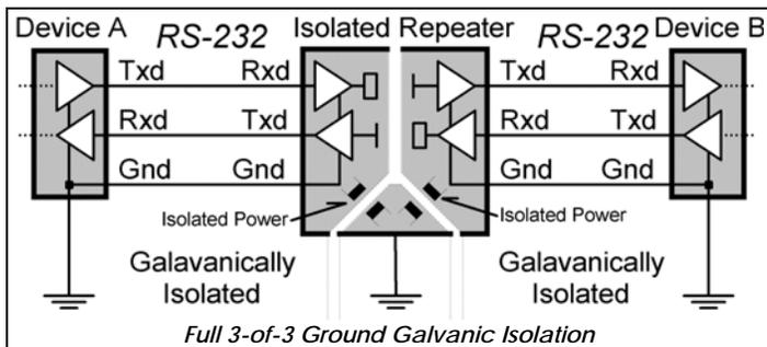
3-port isolation allows a natural physical arrangement where a computer (device A) is located in the control room, the isolated repeater is located in marshaling panels, and the
