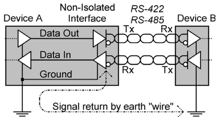
*"Proper operation of the generator and receiver circuits requires the presence of a signal return path between the circuit grounds of the equipment at each end of the interconnection. The circuit reference may be established by a third conductor connecting the common leads of devices, or it may be established by connections in each using equipment to an earth reference."*
