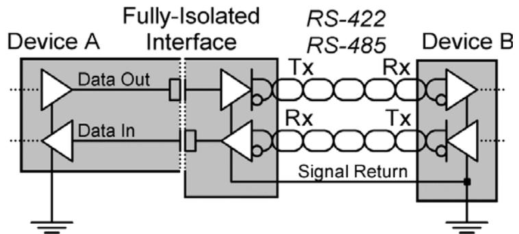
Since we no longer have a signal return path through the earth "wire", full galvanic isolation requires a physical wire to act as a circuit ground. While from an installation stand-point this can be an unexpected cost and even a nuisance, one must consider the trade-offs involved. A properly isolated RS-422/485 system will be almost as effective as fiber optics with none of the technical difficulties of managing fiber cables and connectors.
