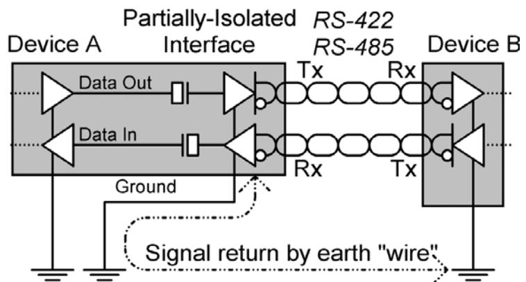
the delicate, high-speed CMOS circuits used in most intelligent devices today. From a surge stand-point, RS-422/485 interface chips are an order of magnitude more robust than - for example - a Pentium CPU or ultra low-power hard disk controller.
