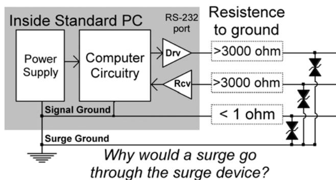
common mode surges. Plus surge diodes can add from 500 to 1000pf per wire -- remember RS-232 requires less than 2500pf per wire. Unless you can identify specific noise sources that would create normal mode spikes on your RS-232 wires, it may not be worth the signal distortion added by surge devices. If noise spikes are a real serious site problem, then you would be better off using a more robust standard like RS-422, modems with transformer isolation, or even fiber optics.
