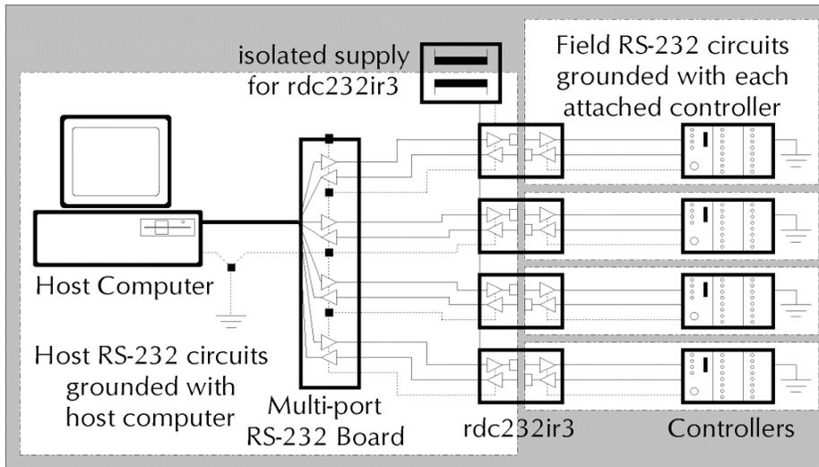
Here is a common installation of RS-232 isolated repeaters (like the rdc232ir) with 2-port galvanic isolation. A small power supply with 1Kv isolation powers the four repeaters. Since all four host RS-232 circuits share a common ground within the computer, any concern about devices
