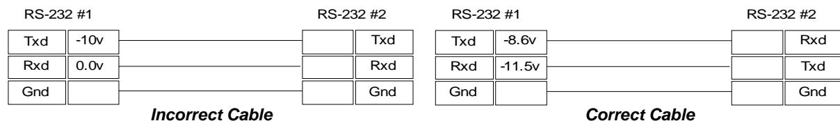
In the drawing at the right - ***the correct cable connected*** - we can see that each transmitter is correctly connected to one receiver. The -8.6vdc (with reference to the common Gnd pin) is the output of transmitter #1 given the load placed on it by receiver #2, and the -11.5vdc is the output of transmitter #2 given the load of receiver #1.
