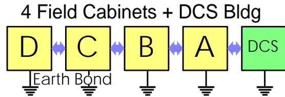
slaves in 4 out-buildings. The overall length was a modest 600 meters. Since every device was grounded to the earth-bonding system, they ran only 2-pair cable with no 5<sup>th</sup> ground wire. An unremarkably design like this with reasonable length and number of slaves should be working fine.
