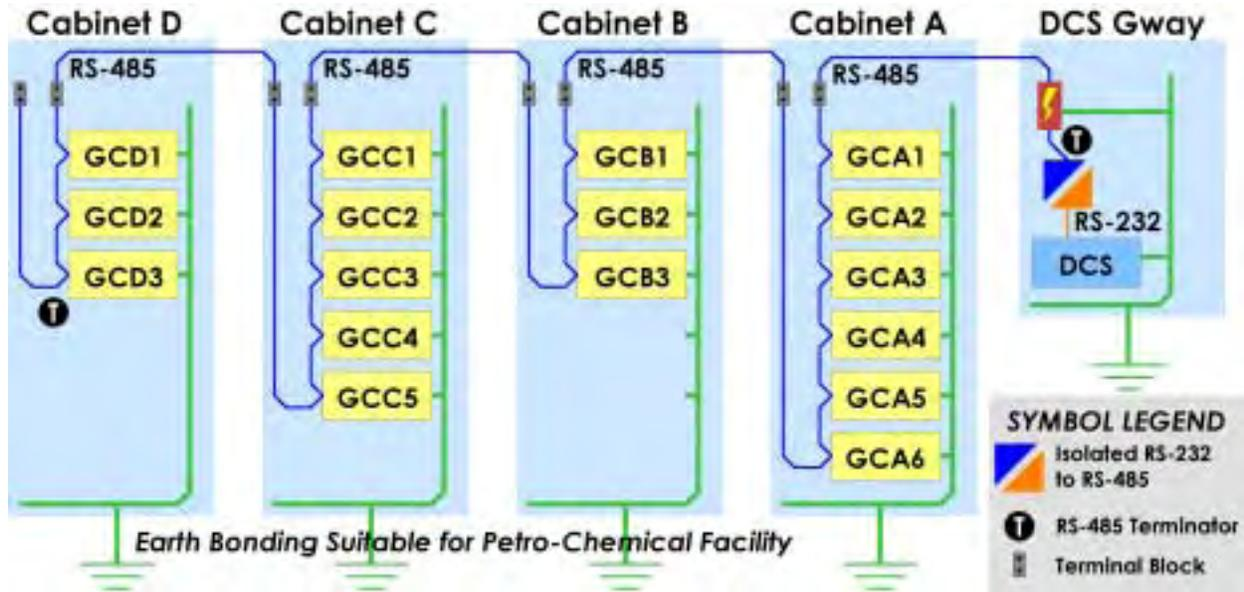
The original design has all of the devices on a single RS-485 network. Only the DCS gateway device is well designed with appropriate surge protection. The original design has no surge protection in the field cabinets. Below is a quick analysis of the “Robustness Factors” (N/C means we don’t plan to change or No-Change). We have 18 devices on one 600m RS-485 bus. Every wire has about 72 points for mechanical failure – meaning the 4-wire RS-485 network has almost 300 screws to come loose.
